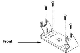
Install the gimbal bracket. Orient the bracket so the arms slope toward the front of your unit.
